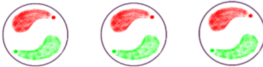
Standard injection pattern 2 nozzle operation
