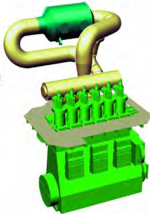
Sulzer 6RTA52U with SCR system
