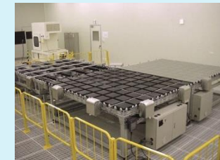
Air-suspended conveyors for large panels
