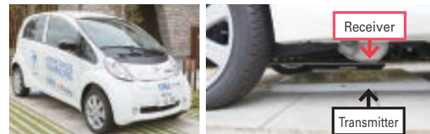
Wireless charging test at Mitsui Home's MIDEAS Experimental House (photo courtesy of Mitsui Home)
