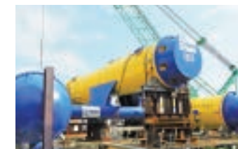
Demonstration machine Kairyu mounted on barge for transportation use
