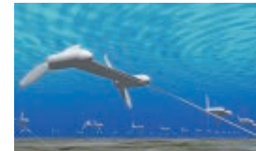
Picture of underwater installation of floating-type ocean current power generation system
