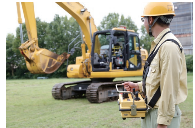
Robo QS (simple remote control system) installed in backhoe
