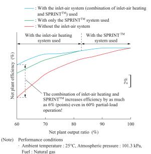
Net plant efficiency under a partial load
