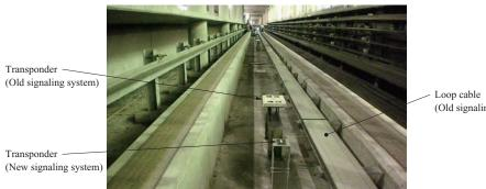
Fig. 2 Trackside equipment for new and old signaling systems
