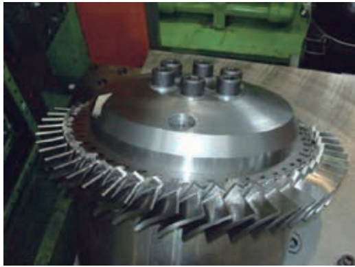
Fig. 10 Compressor blisk manufactured by LFW (3)
