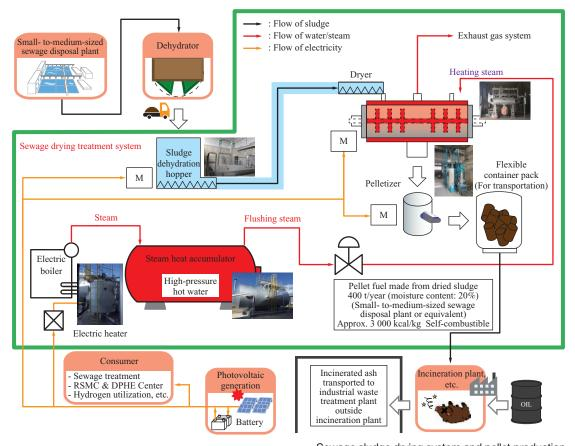
Sewage sludge drying system and pellet production
