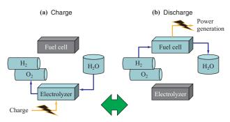
Fig. 4 Charge and discharge behavior of on-board RFC
