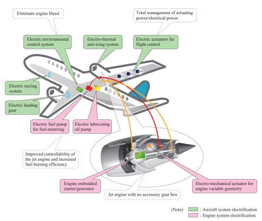
Fig. 1 Overview of the All-Electric Aircraft system
