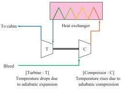
Fig. 2 Outline of air-conditioning using ACS
