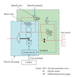
Fig. 5 Schematic of electrical fuel system
