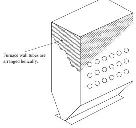
Helical structure in the lower part of the furnace
