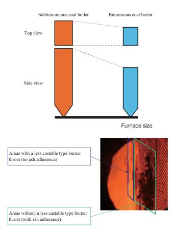
Example of application of a less castable type burner throat
