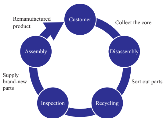
Turbochargers recycling cycle diagram
