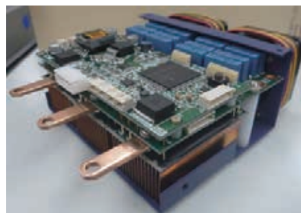
Compact, lightweight inverter (with an output of 35 kW, volume around 500 cc, and mass around 660 g)
