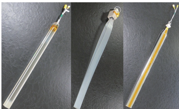
Left: Total absorption calorimeter sensor (lead-tungstate crystal scintillator) Middle: Imaging calorimeter sensor (scintillation fiber) Right: Charge detector (plastic scintillator)
