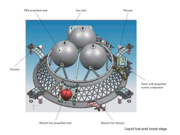
propellant rocket, it has become possible in the final stage to perform fine adjustment for placing a satellite into orbit.
