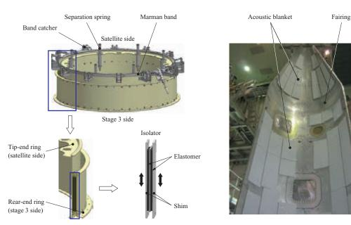
(a) Satellite separation unit (PAF) vibration suppression mechanism
