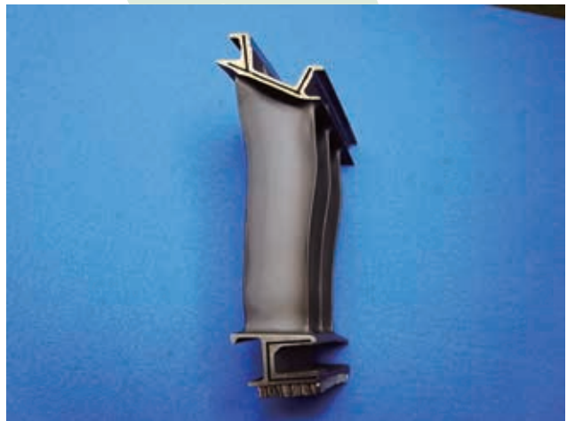
Component made with electrical discharge machining
