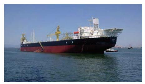
"ERAWAN 2" a floating storage and offloading system
