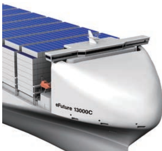
Fig. 6 Forward bridge and front bonnet
