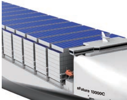
Fig. 10 Arrangement of photovoltaic panels
