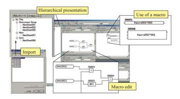
Fig. 4 Control logic editor (LogiCAD)
