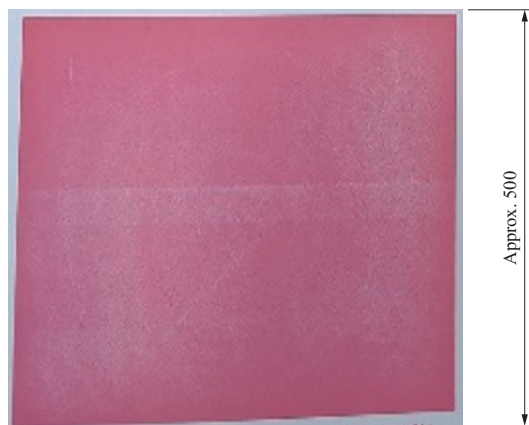
Fig. 10 Surface pressure distribution measurement by pressure-sensitive paper (unit : mm)
