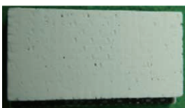
Fig. 11 Comparison of CMC shroud after the test with before the cyclic thermal test
