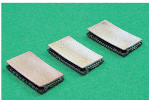
Fig. 16 CMC shrouds after the engine test
