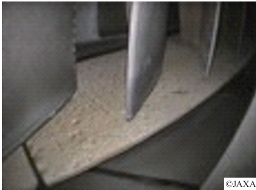
Fig. 14 CMC shroud observed with a borescope
