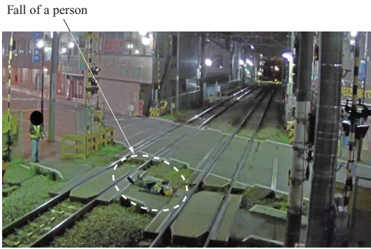
Fig. 13 State of falling down detecting test in on-site level crossing
