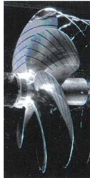
Fig. 7 Observation of propeller cavitation in cavitation tunnel
