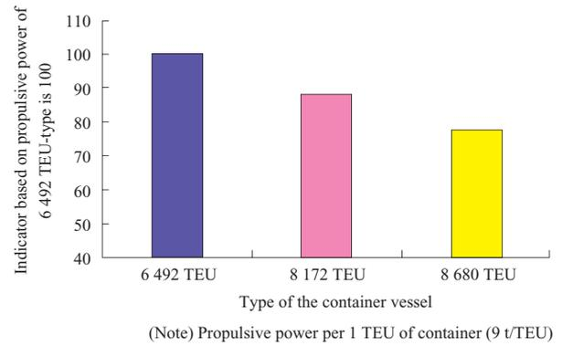
Fig. 3 Mega carrier characteristics compared with previous vessels
