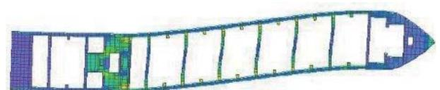
Fig. 11 Deformation by torsional bending moment
