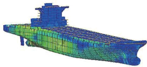
Fig. 13 Extensive structural analysis by SPB-HULL
