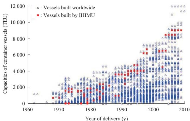
Fig. 1 Delivery of container vessels and sizes
