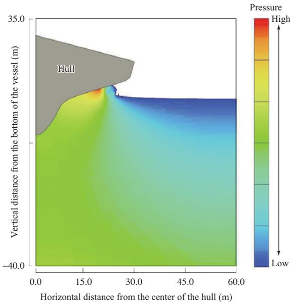
Fig. 12 Pressure distribution on bow flare
