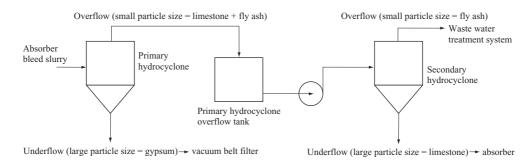
Fig. 6 Principle of two-stage hydrocyclone classifier
