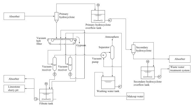
Fig. 5 Process flow of gypsum dewatering system
