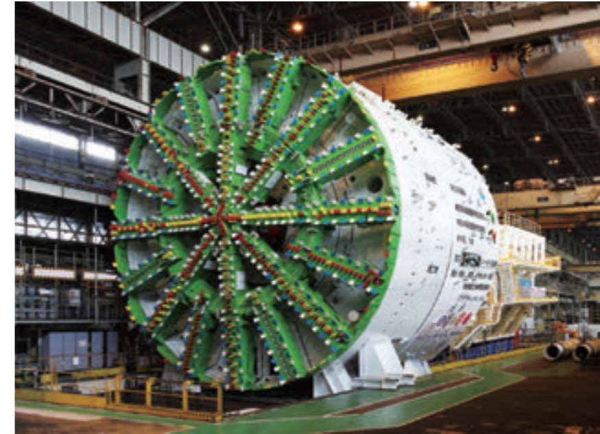
Large-diameter shield tunneling machines
