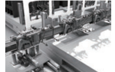
Retrofitting for conveyors between presses
