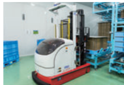
Laser guided forklifts
