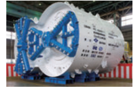
Special section (double-o tube) shield tunneling machines
