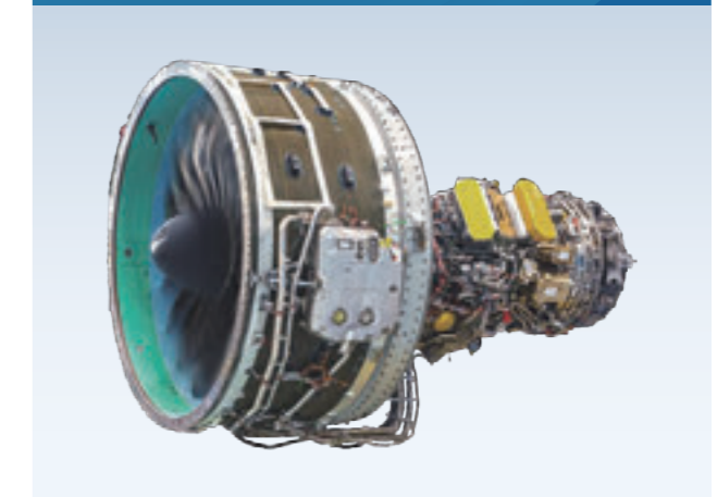
PW1100G-JM turbofan engine mounted on Airbus A320neo (photo courtesy of JAEC)
