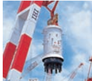
Reactor pressure vessel
