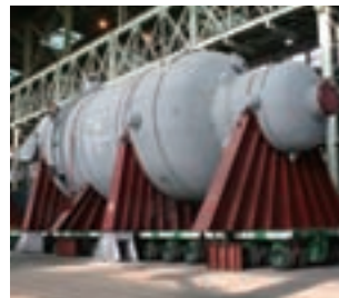
Ethylene oxide reactor
