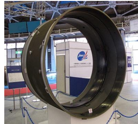
Fan case of PW1100G-JM, to be produced at the Tomioka Works, IHI Aerospace Co., Ltd. (provided by Japanese Aero Engines Corporation)
