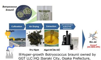
IHI and New Energy and Industrial Technology Development Organization are proceeding with the technology development for production of bio-jet fuel from microalgae. Regarding to the bio-jet fuel produced by this technology, IHI has acquired the international standard for alternative jet fuel for aviation "ASTM D7566 Annex 7".
