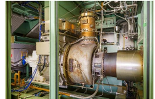
Liquid ammonia and natural gas co-fired 2,000-kilowatt-class gas turbine at IHI's Yokohama Works
