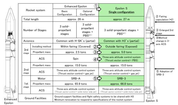
(\*1) PBS (Post Boost Stage): liquid propellant gas jet system to increase orbit injection accuracy
