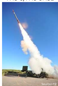
Type-11 surface-to-air missile/ Surface-to-air guided missile for base air defense
