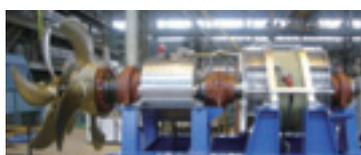
The two liquid nitrogen cooled superconducting motors and the counter rotation propeller system at the exhibition in 2008
