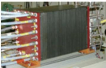
Prototype of a regenerative fuel cell
