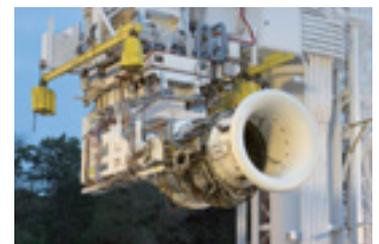
The *CF34-10A* undergoing ground tests
