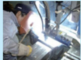
MIG welding using coaxial hybrid solid wire
