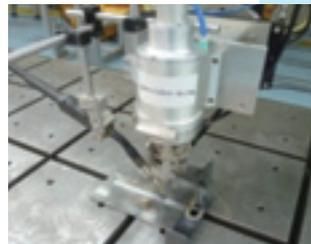
Laser-arc hybrid welding head
