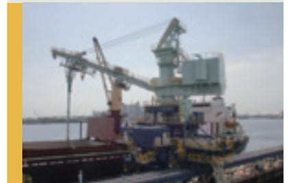
The new pneumatic unloader at Chiba Kyodo Silo Co., Ltd.
