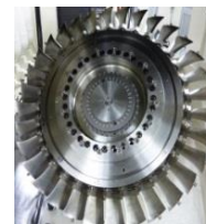
Automated integrated bladed rotor line for PW1100G-JM engine
