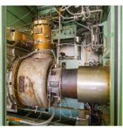
Liquid ammonia and natural gas cofired 2,000-kilowatt-class gas turbine at IHI's Yokohama Works
