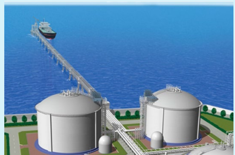
Illustration of large ammonia receiving terminal
