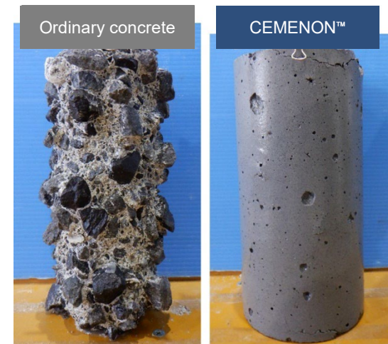
<Comparison of acid resistance of ordinary concrete and CEMENON™>
