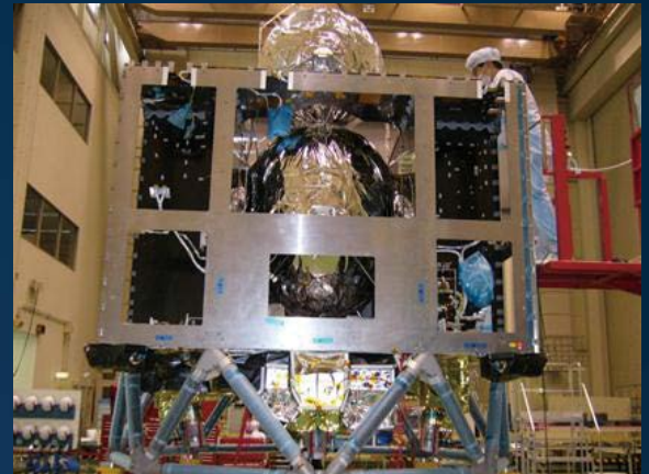
Unified Propulsion System (SELENE)
