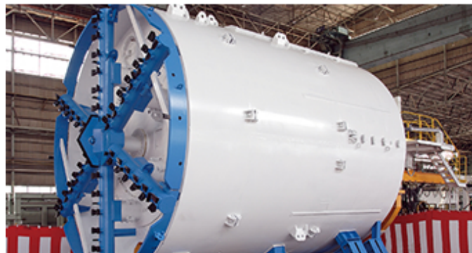
Tunnel boring machine for use in Jakarta
