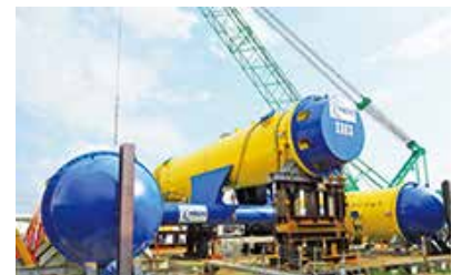
Demonstration machine Kairyu mounted on barge for transportation use
