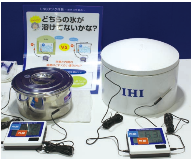
Hands-on model fabricated with insulating material used in LNG tanks
