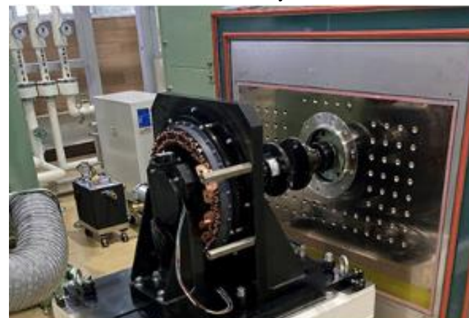
Fig.2 A prototype of a 250-kW high-power electric motor ©Akita Prefectural University
