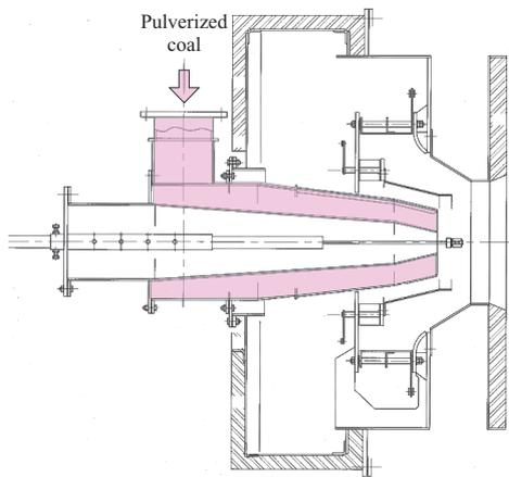
Fig. 10 Pulverized coal burner (IHI-DF burner)
