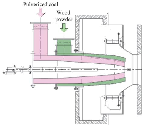
Fig. 13 Burner for wood powder and pulverized coal
