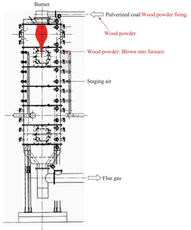
Fig. 1 Small-scale combustion test facility
