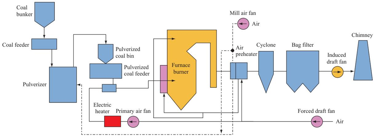
Fig. 3 Large-scale combustion test facility
