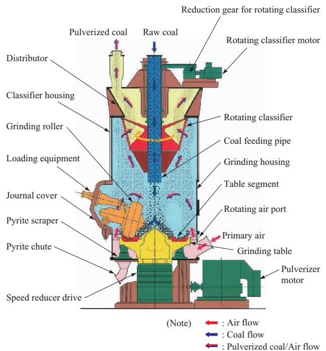
Fig. 4 Coal pulverizer
