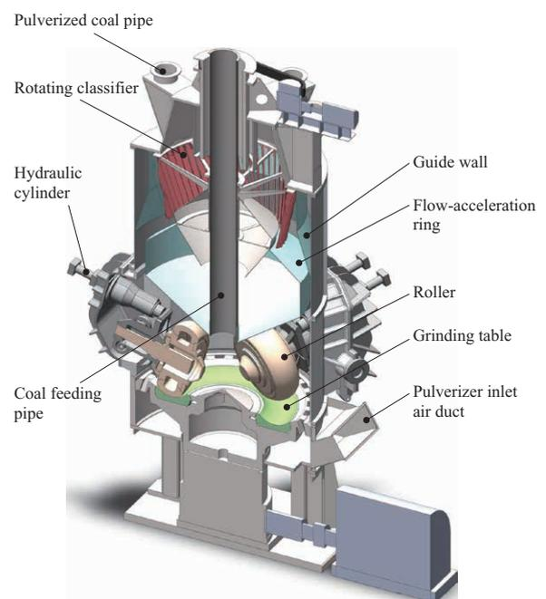
Fig. 8 Wood pellet pulverizer
