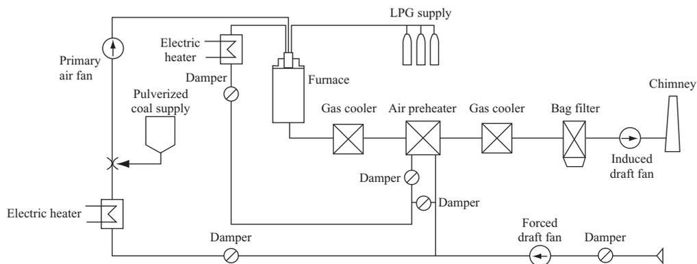
Fig. 2 Schematic diagram of combustion test facility
