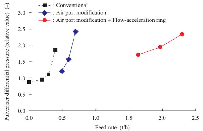
Fig. 7 Increasing wood pellet grinding capacity
