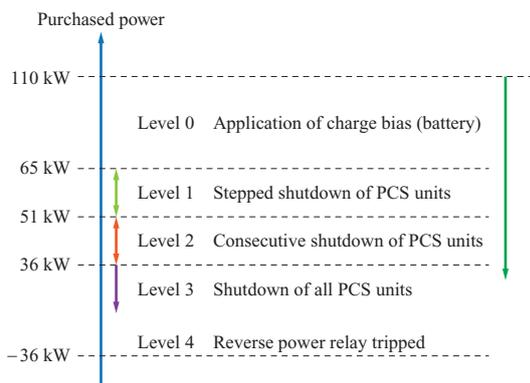
Fig. 5 Settings to prevent backfeeding
