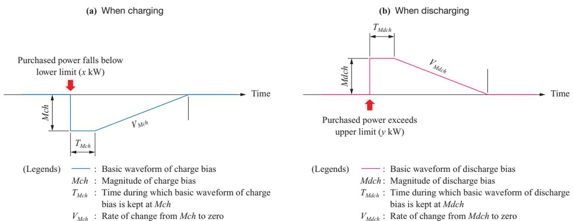
Fig. 6 Basic waveform for charging/discharge bias — under charging
