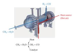
Compact reactor as Steam Methane Reformer (SMR) for hydrogen production
