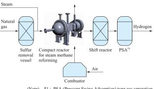
(Note) \*1 : PSA (Pressure Swing Adsorption) type gas separation and refinement equipment
