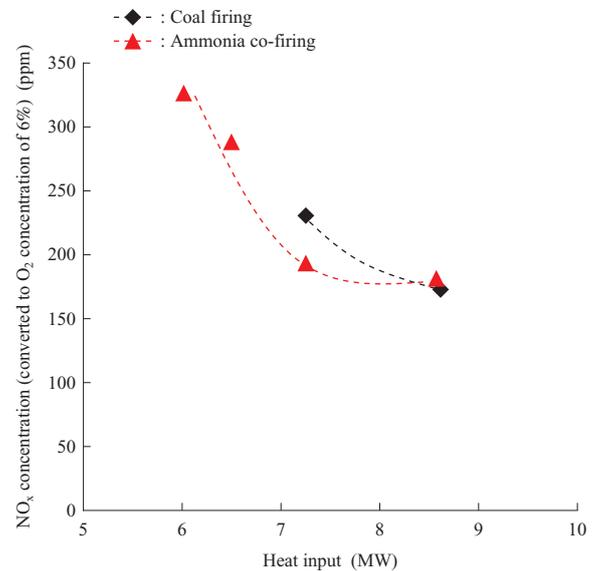
Fig. 8 Relationship between heat input and NO<sub>x</sub> concentration
