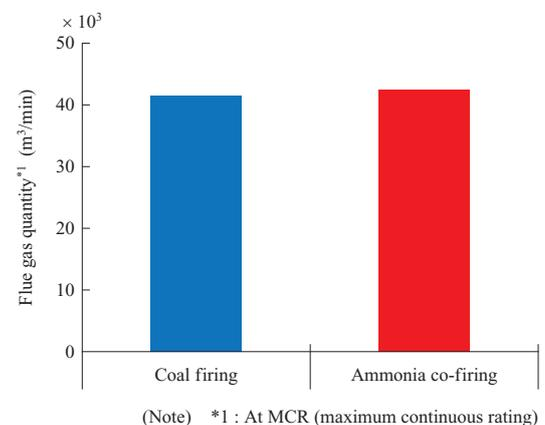
**Fig. 14** 1 000 MW-class boiler exhaust gas volume
