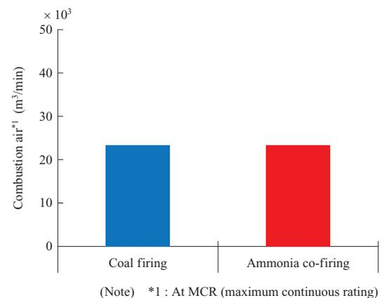
**Fig. 13** 1 000 MW-class boiler\_combustion air
