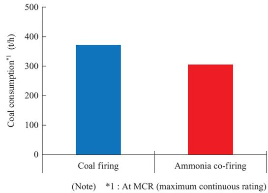
**Fig. 12** 1 000 MW-class boiler\_fuel consumption
