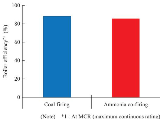
**Fig. 11** 1 000 MW-class boiler\_boiler efficiency
