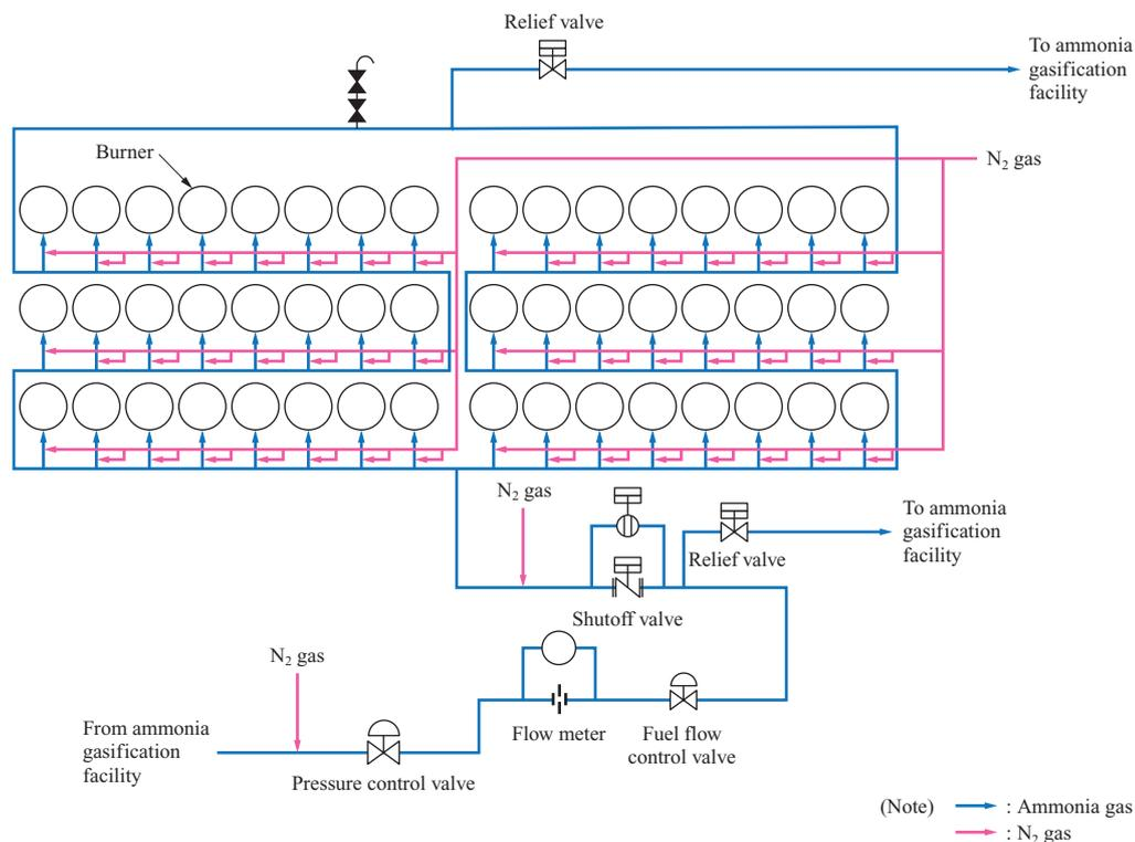
Fig. 16 Schematic diagram of 1 000 MW-class boiler\_ ammonia gas system
