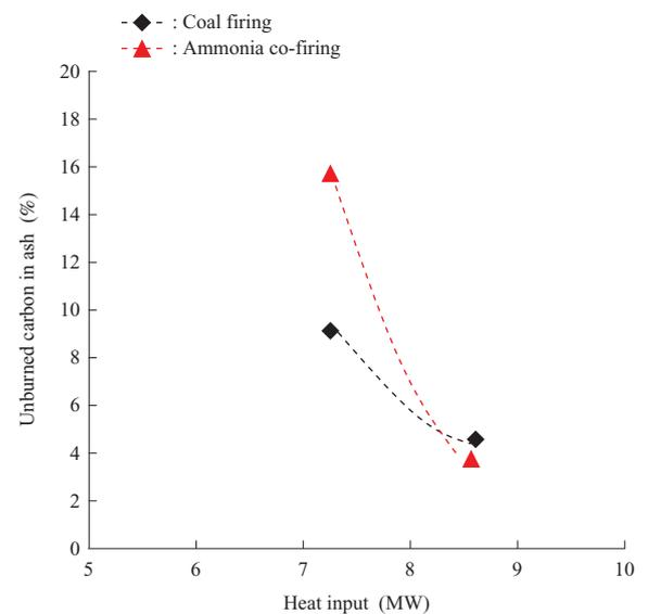
Fig. 9 Relationship between heat input and unburned carbon
