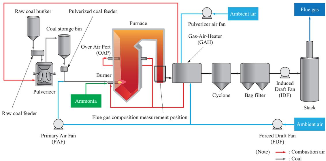
Fig. 2 Main diagram of test furnace
