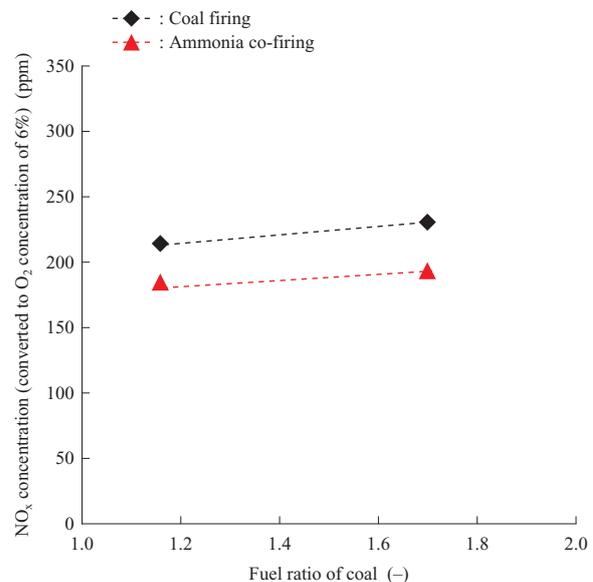
Fig. 10 Relationship between fuel ratio and NO<sub>x</sub> concentration
