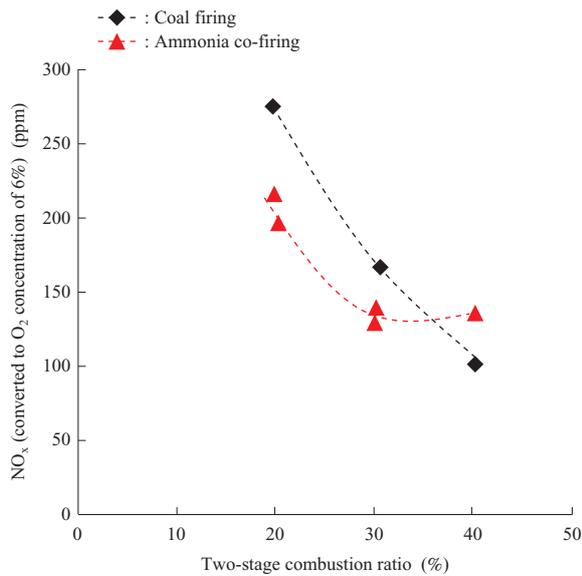
Fig. 6 Relationship between two-stage combustion ratio and NO<sub>x</sub>
