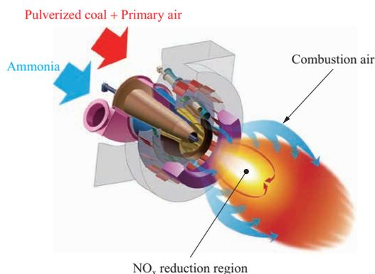
**Fig. 3** Enlarged view of burner used in co-firing experiment
