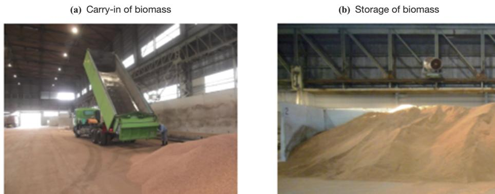
Fig. 4 Biomass carry-in and storage for the demonstration tests
