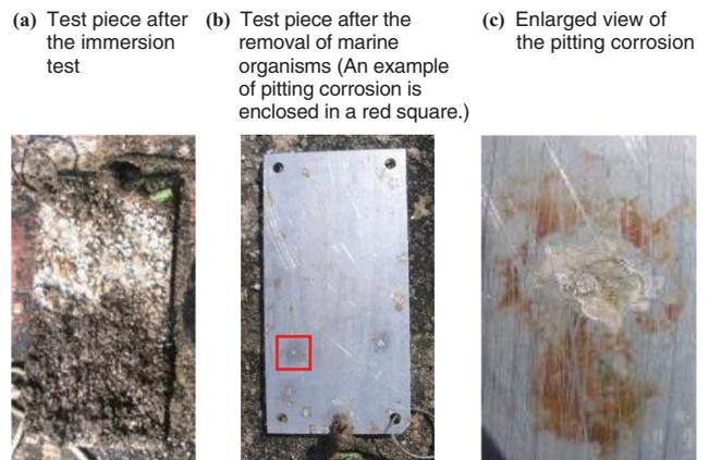
**Fig. 7** Sea immersion result of SUS304 test piece
