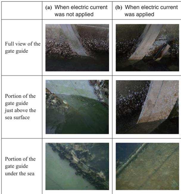
**Fig. 5** Result of immersion test after application of weak electric current anti-biofouling method for one year
