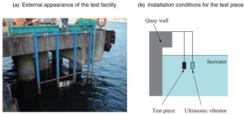
Fig. 10 Ultrasonic system test environment
