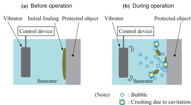
Fig. 9 Principle of ultrasonic anti-biofouling method
