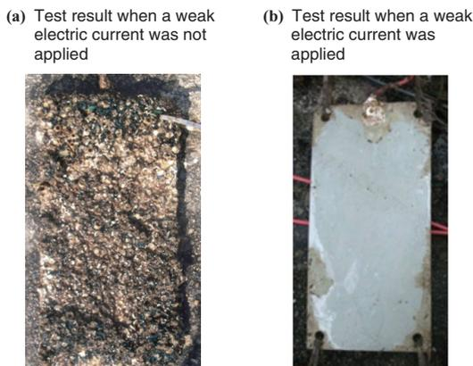
Fig. 3 Result of immersion test for weak electric current anti-biofouling method during breeding season of attached organisms
