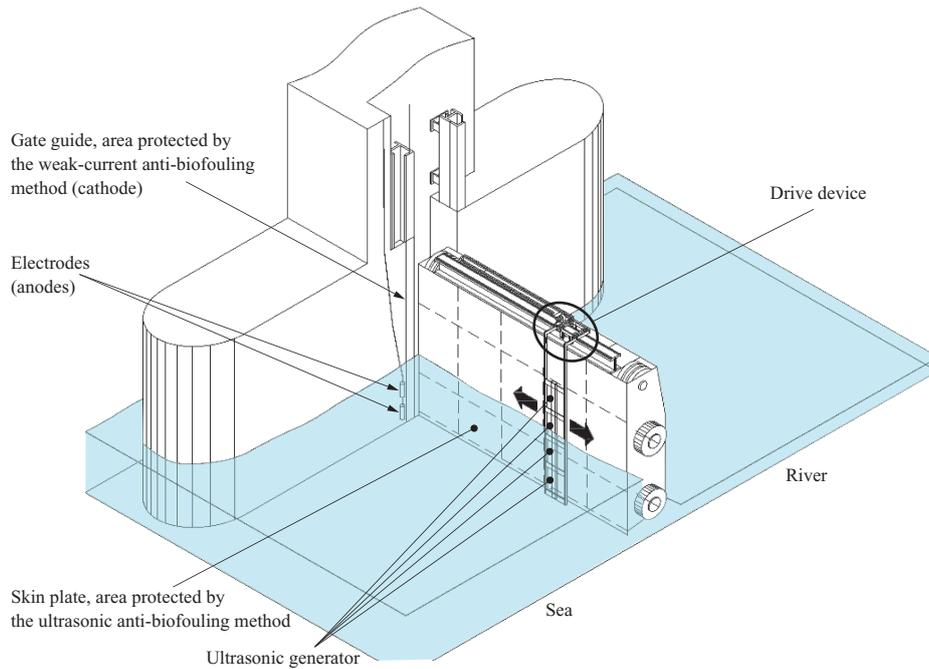
Fig. 1 Conceptual image of application of anti-biofouling method for roller gates
