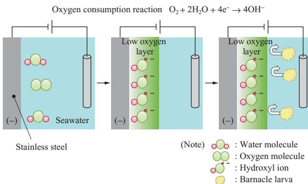
Fig. 2 Principle of weak electric current anti-biofouling method
